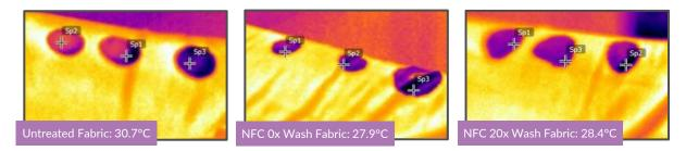
When moisture is absorbed into the fabric, it provides an immediate cooling effect that is caused through an endothermic reaction.
